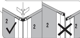
► Adjust the two doors with the screws located on the upper rollers so doors to fit together perfectly.
