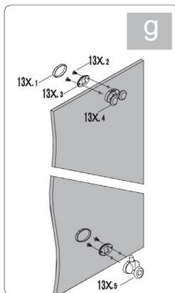
► Place the sealing rubbers, profiles with magnets, and the rollers.
