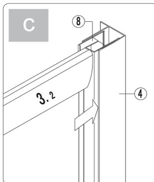
► The recess must be on the inside as on the drawing.
