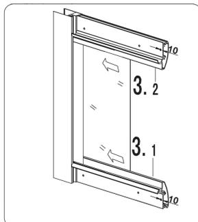
► Screw the horizontal guides to the vertical profile bearing the special recess for stable crystal in order to set up the metal frame.
