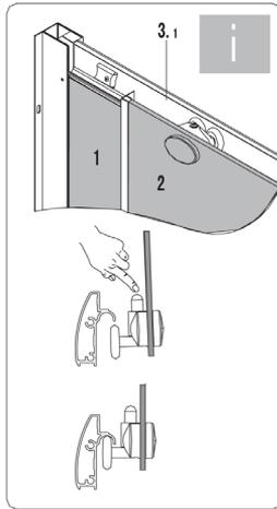
► Hang the doors on the upper guide and lock them by pressing the springs on the lower rollers to apply appropriate and in the lower guide.
