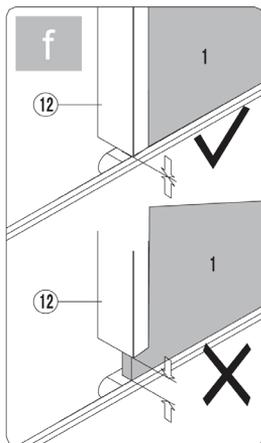
► Insert the sealing profile by pressing it.
