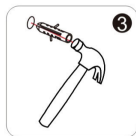
Driving expansion pipe into the wall
