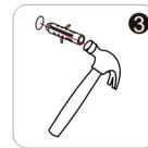
Driving expansion pipe into the wall
